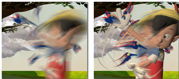
Figure 11: A comparison of conventional motion blur (left) with our weighted motion blur including speed lines (right).
